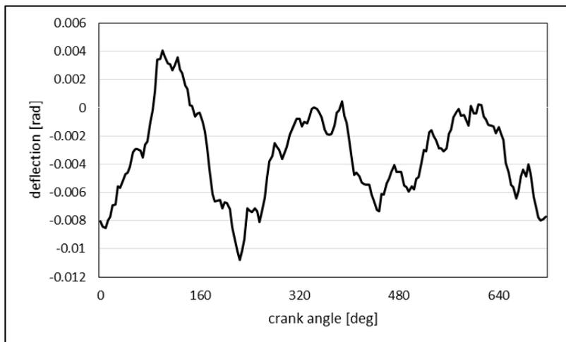
**Fig. 3.** Torsional deflection of the shaft in time of two revolutions (720° CA)
