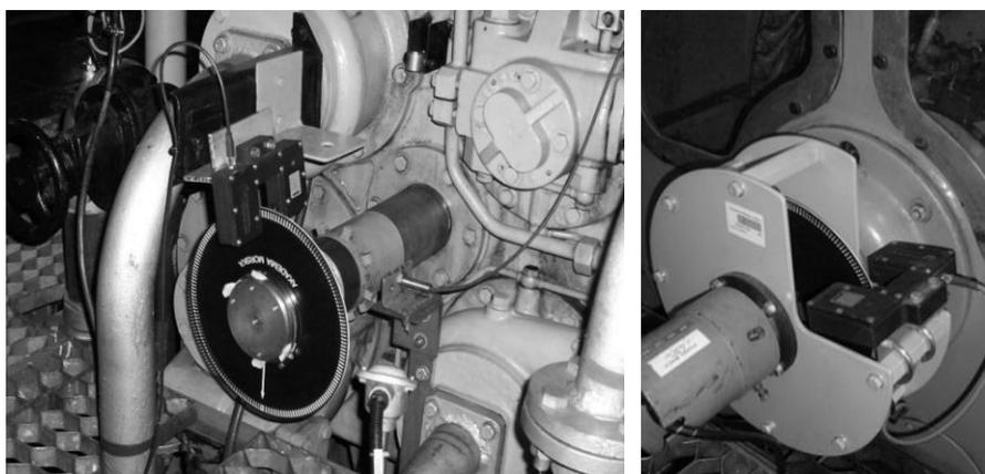
**Fig. 4.** Discs and measuring heads mounted at engine's crankshaft end
