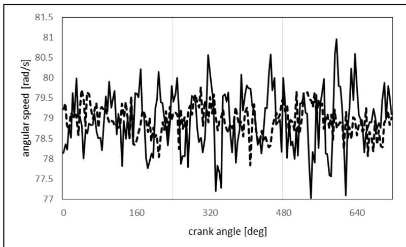
**Fig. 2.** Wavelets of instantaneous angular speed in domain of crank angle. Solid line refers to “master” disc A and dotted one to the disc B
