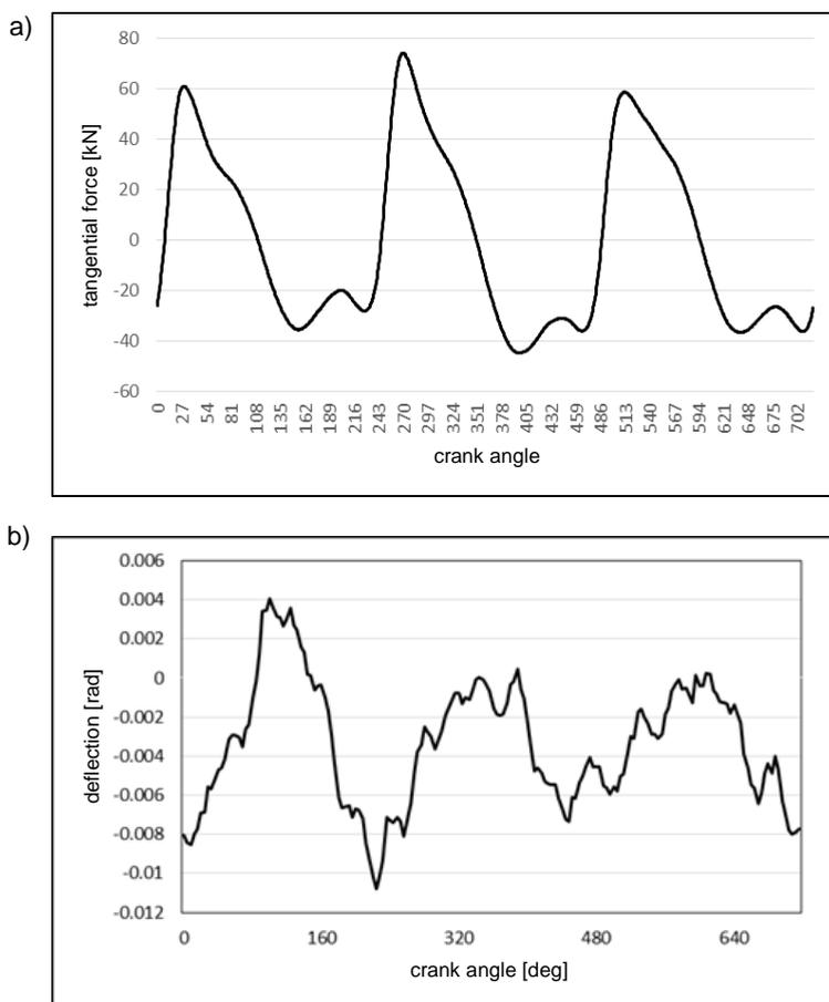
**Fig. 5.** Model of tangential force wavelet of 3-cylinder 4-stroke engine (a) and measured torsion wavelet (b)
