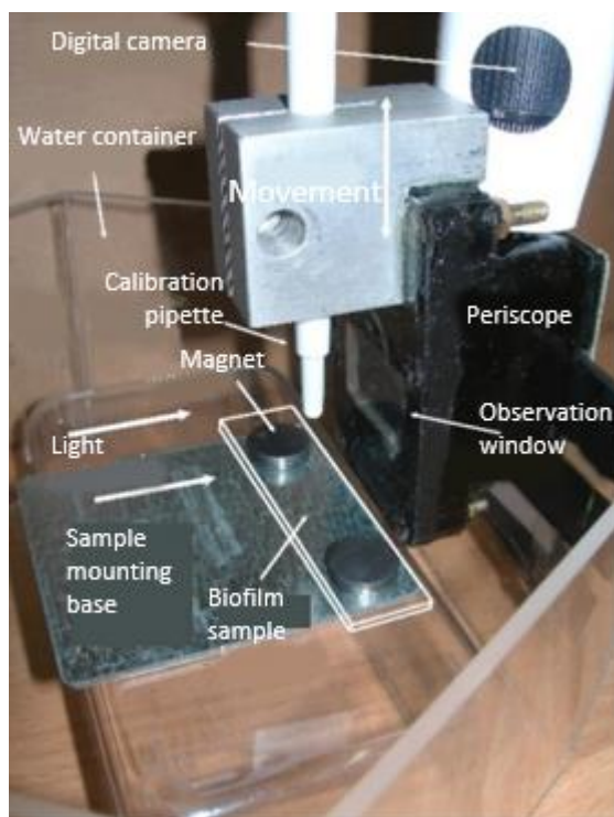
Fig. 6. Experimental set-up for dynamic contact angle determination on submerged solid surfaces designed for field work
